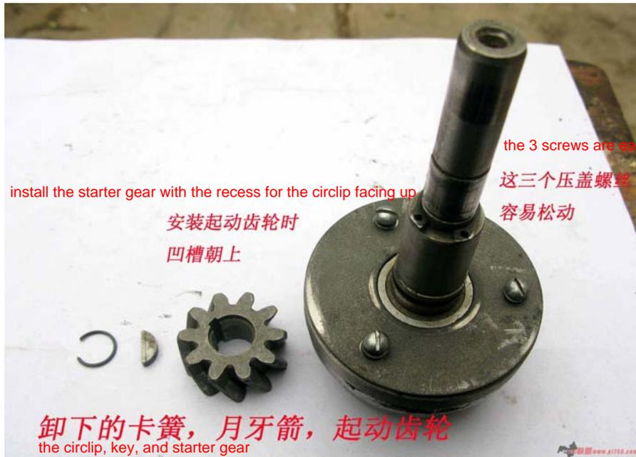
install the starter gear with the recess for the circlip facing up
